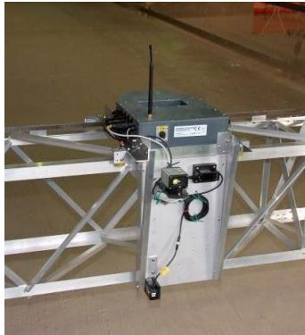
Fig. 23. 2D bed profiling system
