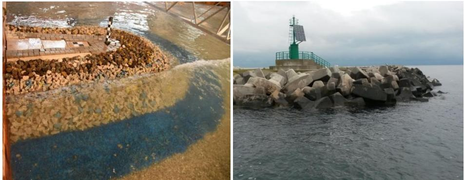
Fig. 20. Roundhead stability 3D test
