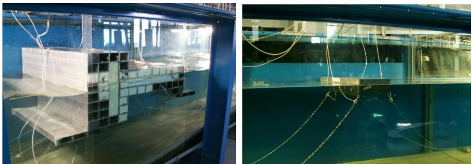
Fig. 6. Floating breakwaters (wave reflection, wave transmission and loads)
