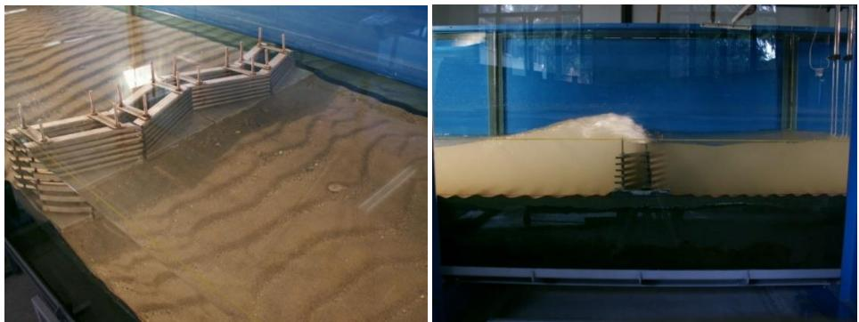
Fig. 12. Coastal protection structure
