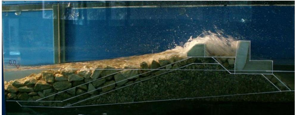
Fig. 5. Overtopping measurements
