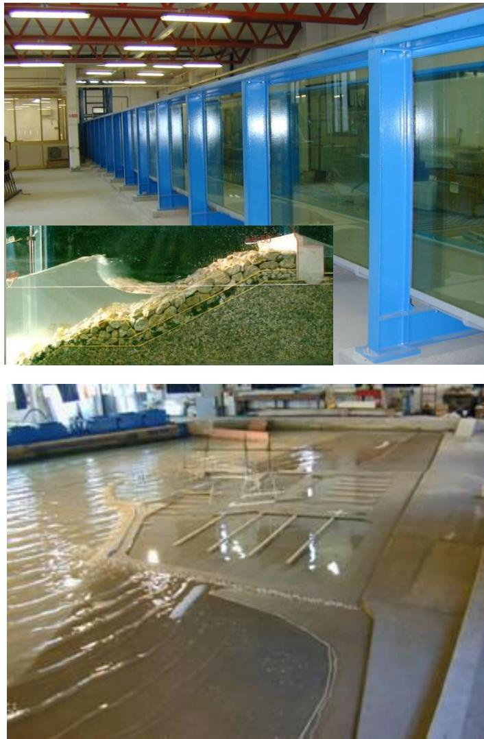
Fig. 1. Wave flume (above), wave basin (below)
