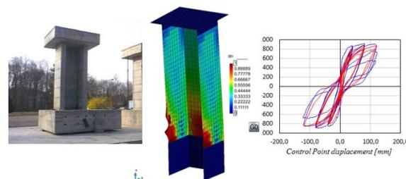
*The validation of the adopted non-linear numerical model (developed by researchers of DICEA) has first been conducted through the reproduction of three experimental tests on complex RC walls found in literature.*
